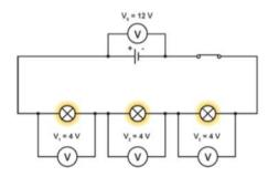
• The total **resistance** in a series circuit is equal to the sum of all the resistances of the components.
