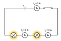
The Voltage in a series circuit splits up amongst the component in the circuit.
