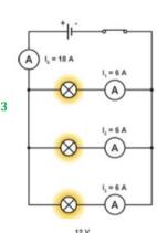
The Voltage supply in a parallel circuit is equal to the voltage in each branch.
