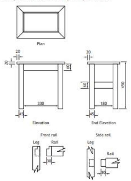
Note: The rails are joined to the legs using the joints shown in the drawings above. All sizes are in millimetres.
